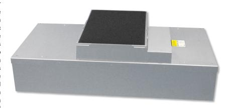
The MAC 10® IQ FFU uses a combination of EC motor technology with ENVIRCO's unique baffling system and forward curve fan to make it intelligent and energy-efficient. The electronically commutated (EC) motor with internal micro-computer provides low energy consumption (235 watts at 90 fpm (0.45 m/s)), high performance and long motor life. The IQ utilizes ENVIRCO's VE5 baffling technology, offering low sound levels that are a MAC 10<sup>®</sup> family benchmark.
