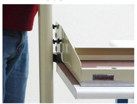
3. Slide the legs to the desired worksurface height while observing the height marking tape.
