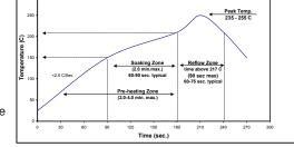
Kester Reflow Profile SnAgCu Alloys
