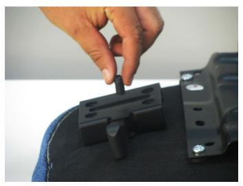
1. Remove the end travel retention pins. Slide out the arm lock cam handle.
