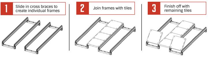
Continue the process to desired width. Use FOUNDATION connectors to join sections end-to-end to desired length.
