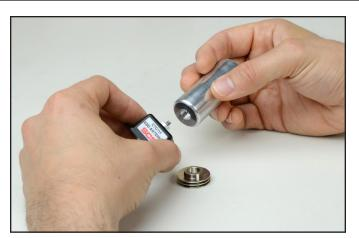
Figure 4. Replacing the standard antenna with the ionizer antenna
