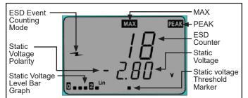
Figure 13. Static Voltage Field channel
