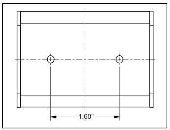
Figure 5. Mounting hole locations on the back of the EM Aware Monitor
