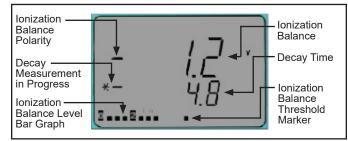
Figure 14. Balance and Decay Mode channel
