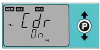
Figure 12. Enabling the noise filter
