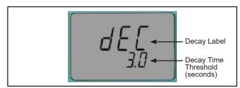
Figure 15. Decay time threshold settings
