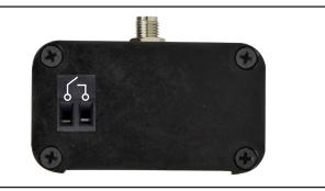
Figure 7. Relay terminal pin-out
