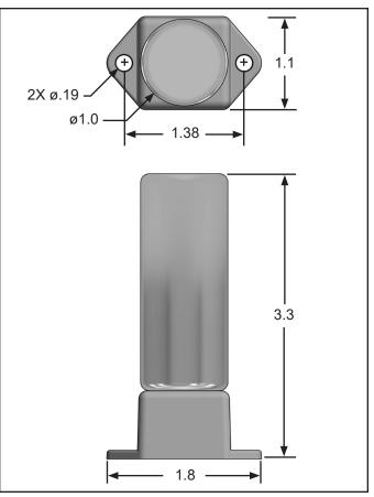
Figure 26. Ionizer antenna dimensions (inches)
