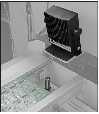
Figure 23. Using the EM Aware Monitor with ionizer antenna on an SMT conveyor with the SCS <u>963E</u> Benchtop Air Ionizer
