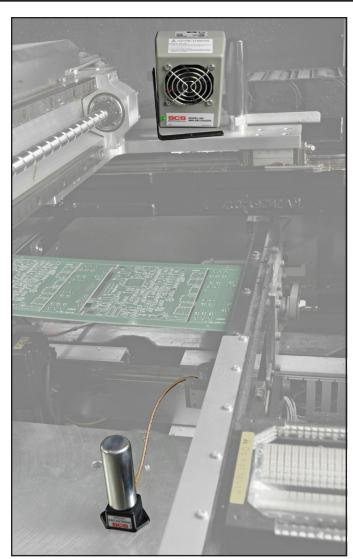
Figure 24. Using the EM Aware Monitor with ionizer atenna inside of a pick-and-place machine with the SCS <u>960</u> Mini Air Ionizer
