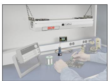
Figure 22. Using the EM Aware Monitor with ionizer antenna on a workbench with the SCS <u>770112</u> Ion Pro™ Overhead Ionizer
