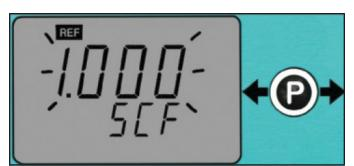
Figure 20. Setting the Smart Coefficient value
