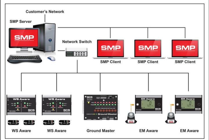
Figure 8. SMP system setup
