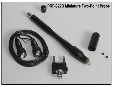
and an insulated test bed. They provide surface resistance measurements in ohms per ESD S11.11 Surface Resistance standard. To estimate ASTM D-257 Surface Resistivity in ohms/square, multiply the fixture measurement by 10, i.e., add one decade. Replaceable conductive electrode Ring and cap sets are available separately to enhance contact resistance on irregular surfaces and composition materials.
