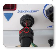
Align guide on connector with slot on power receptacle.
