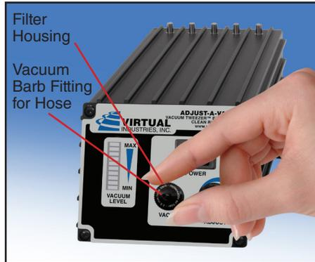
2. Select a probe with a vacuum cup that is slightly smaller in diameter to the outline of the parts that you want to pick and place. Securely install it on the tapered end of the vacuum pen tip. Selecting a vacuum cup that is too large or too small will result in improper operation.
