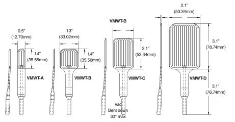
Molded Wafer Tips VMWT-A, VMWT-B and VMWT-C are available with a 10°, 20° or 30° bend in the up or down direction as shown in the left drawing above. To order a tip with the up or down bend, add the angle plus a "U" for up or a "D" for down to the part number. EXAMPLE: Part number VMWT-A20D is a VMWT-A Wafer Tip with a 20 degree bend in the down direction. Custom angles are available upon request. Pricing is as above.
