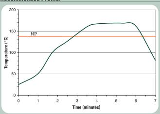
This profile is designed for use with Indalloy®282 and can serve as a general guideline in establishing a reflow profile for use with other alloys. Adjustments to this profile may be necessary based on specific process requirements.
