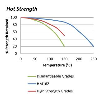
"Hot strength" Breakaway strength on M10 Zinc plated bolts according to ISO 10964. Cured at 23°C for 24 hours then conditioned for 30 minutes at testing temperature.
