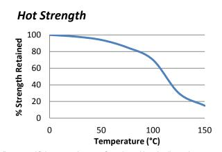
"Hot strength" shear strength tests performed on mild steel. Fully cured specimens conditioned to pull temperature for 30 minutes before testing at temperature. TA435 can withstand higher temperatures for brief periods (such as for paint baking and wave soldering processes) providing the joint is not unduly stressed. The minimum temperature the cured adhesive can be exposed to is -55°C (-65°F) depending on the materials being bonded.
