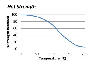
"Hot strength" shear strength tests performed on mild steel. Fully cured specimens conditioned to pull temperature for 30 minutes before testing at temperature. TA436 can withstand higher temperatures for brief periods (such as for paint baking and wave soldering processes) providing the joint is not unduly stressed. The minimum temperature the cured adhesive can be exposed to is -55°C (-65°F) depending on the materials being bonded.
