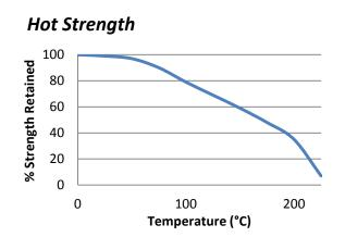
"Hot strength" shear strength tests performed on mild steel. Fully cured specimens conditioned to pull temperature for 30 minutes before testing at temperature. TA437 can withstand higher temperatures for brief periods (such as for paint baking and wave soldering processes) providing the joint is not unduly stressed. The minimum temperature the cured adhesive can be exposed to is  $-55^{\circ}C$  ( $-65^{\circ}F$ ) depending on the materials being bonded.
