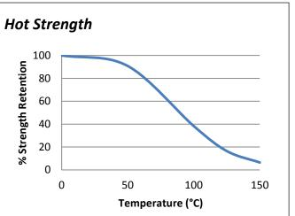
TA4820 can withstand higher temperatures for brief periods (such as for paint baking and wave soldering processes) providing the joint is not unduly stressed. The minimum temperature the cured adhesive can be exposed to is -40°C (-40°F) depending on the materials being bonded.
